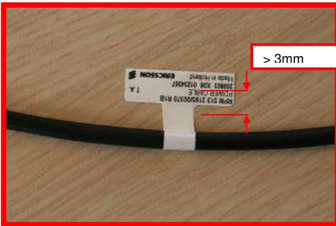
Gap between label and cable is greater than 3mm.
