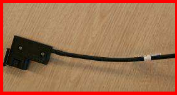
Label is not positioned at 12 o'clock
