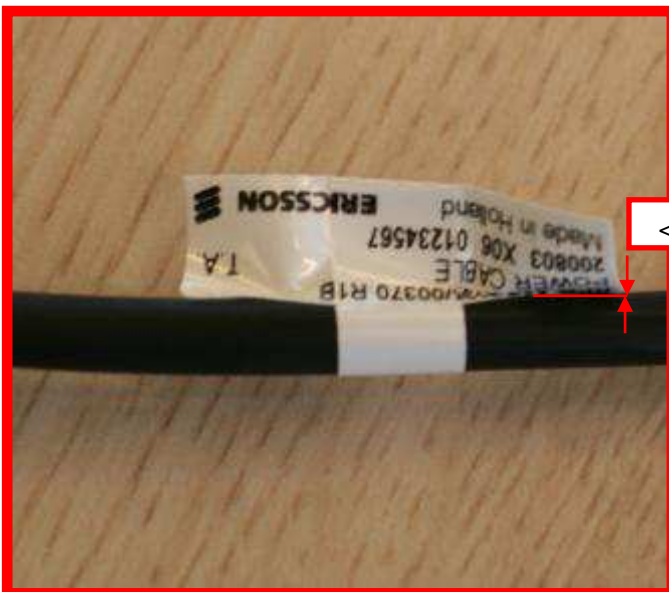
Gap between label and cable is less than 1mm.
