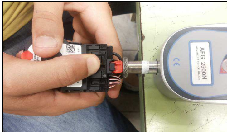
Photo 8 - CPA actuation with the locked housing
