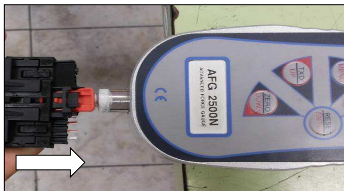
Photo 16 - Connector insertion force to counterpart
