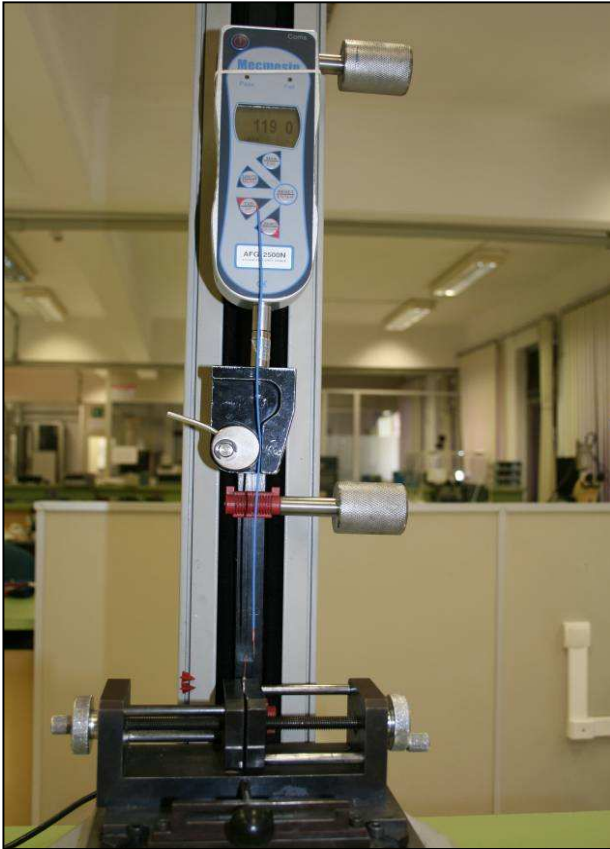
Photo 18 - Crimp pull-out test
