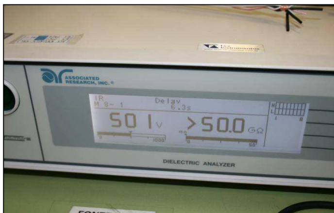
Photo 12 - Voltage applied (500Vdc)
