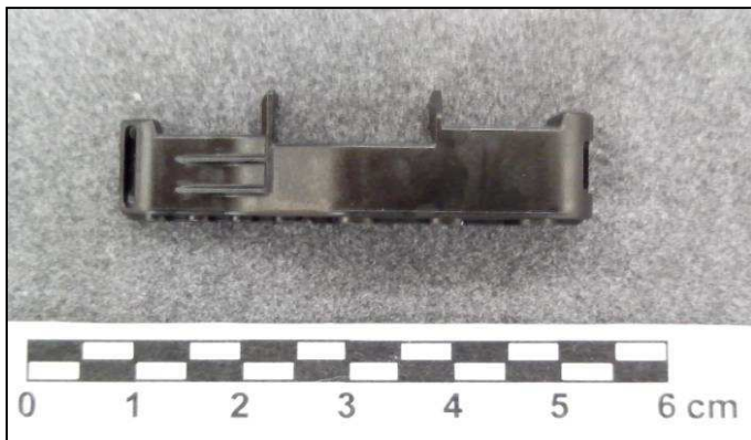
Photo 3 - WIRE DRESS, 7 POSN.,MCP/QQS, REC. PN: 2133881-1
