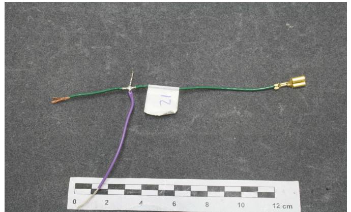
Picture 12: Combination XII - AVSSB 0,50mm 2 (Sumitomo terminal / Sumidenso Process)
