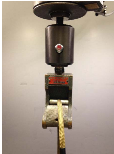
Figure 15 – Cable Clamp On Crosshead
