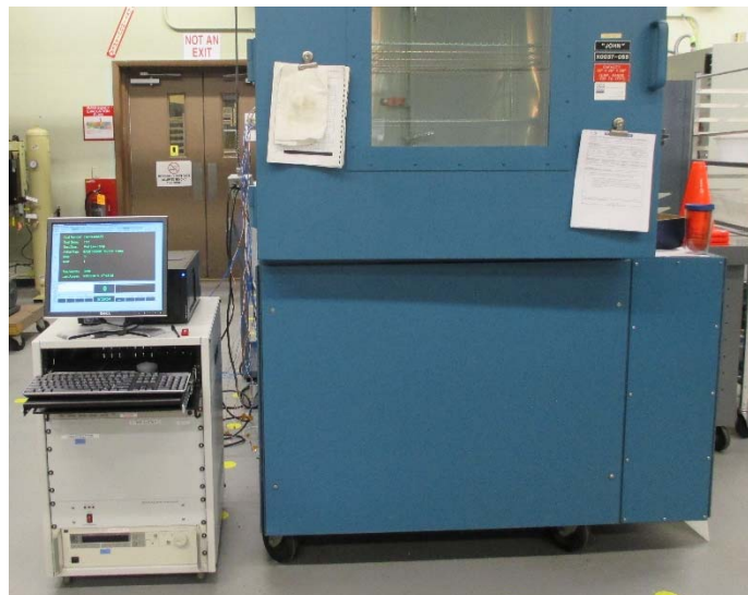
Figure 11 – Voltage Drop Measurement Setup in Chamber Test Group 3
