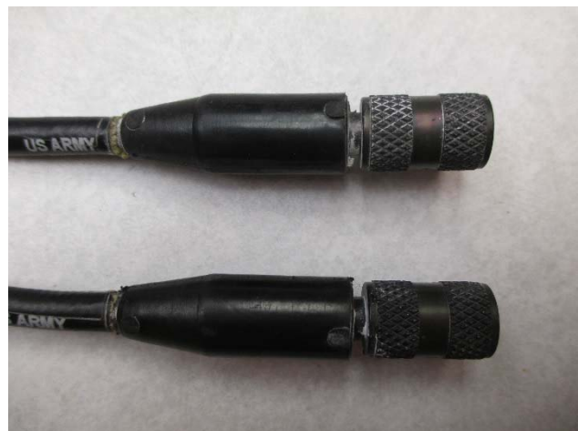
Figure 8 – White Residue on Receptacles Test Group 5
