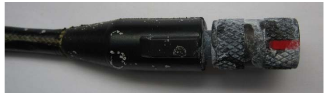
Figure 6 – Specimen 402 Receptacle Post Salt Spray
