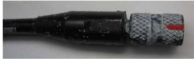
Figure 4 – Specimen 401 Receptacle Post Salt Spray
