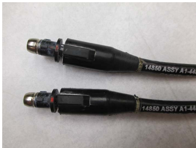
Figure 7 – White Residue on Plugs Test Group 5
