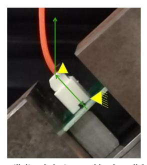
2. The force of post contact will directly be impacted by the pull force direction because of the force-lever of header housing & PCB, so, on this point we tested the force by two directions: 90° vertical & 45° slant as the data shown above.
