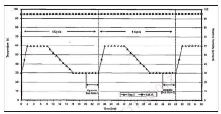
Figure 2 - Humidity Test Chamber Profile
