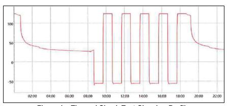
Figure 1 - Thermal Shock Test Chamber Profile
