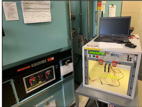
Figure 27 – IR at Elevated Temperature Test Set Up
