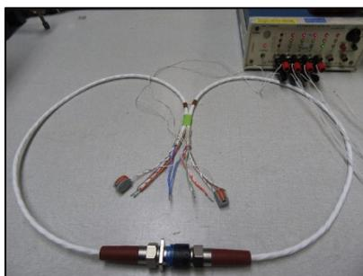
Figure 14 – Electrical Engagement Test Set Up
