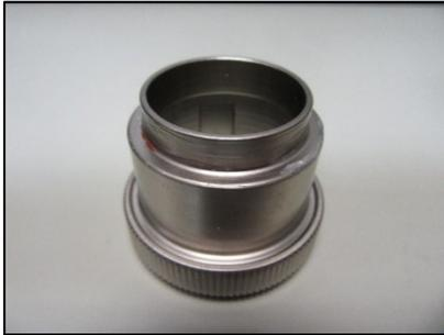
**Figure 17 –Back Shell without Rear Seal**
