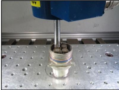
**Figure 18 – Insert Retention Test Size 25, Towards Rear**
