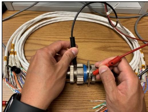
Figure 11 – Shell to Shell Conductivity
