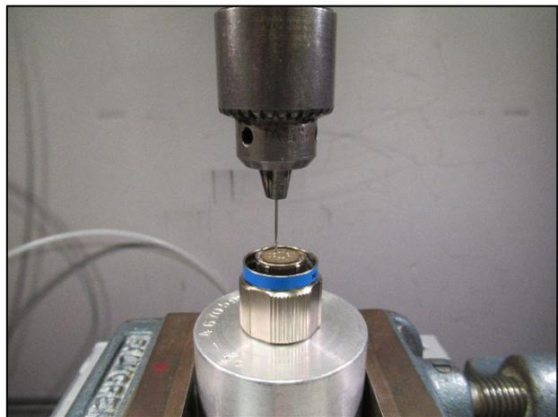
Figure 26 – Typical Contact Retention Setup Plug
