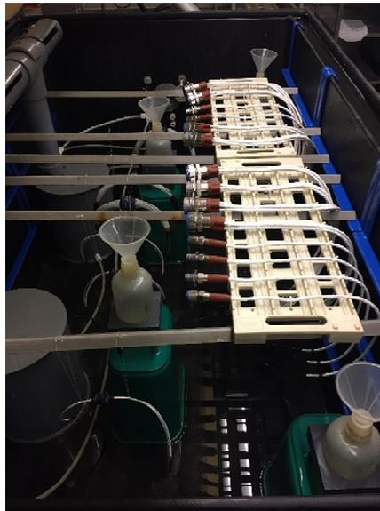
**Figure 12 – Salt Spray Test Set Up**
