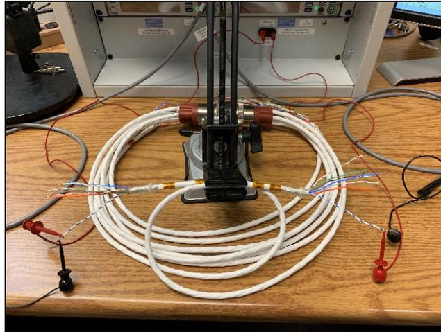
Figure 13 – Low Level Contact Resistance Test Set Up
