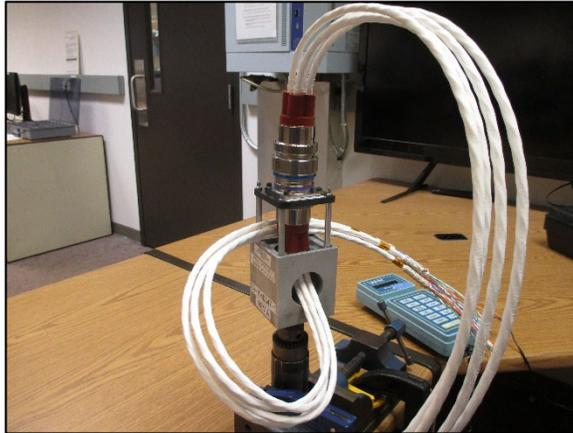
Figure 4 – Typical Coupling Torque Test Set Up
