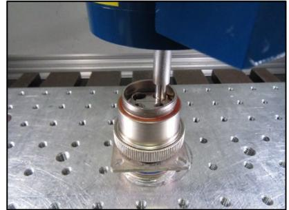
**Figure 19 – Insert Retention Test Size 25, Towards Front**
