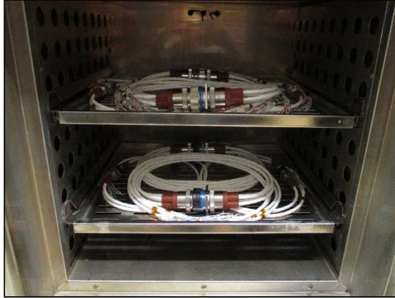
Figure 30 – High Temperature Exposure Test Set Up
