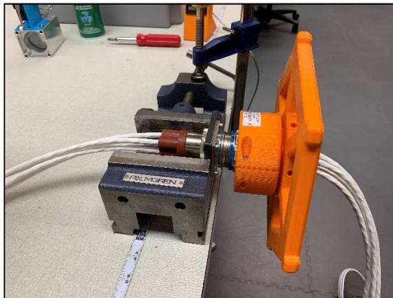
Figure 5 – Durability Test Set Up
