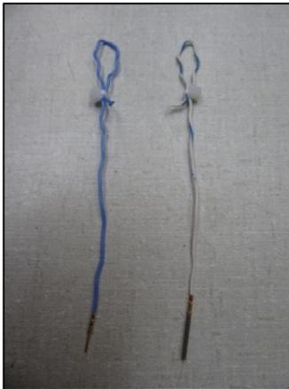
Figure 1 – Pin/Socket Assmely
