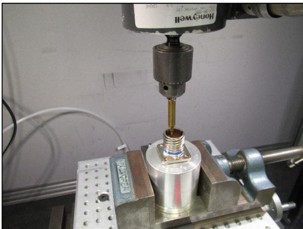
Figure 25 – Typical Contact Retention Setup Receptacle
