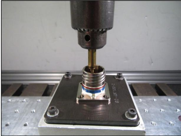
Figure 23 – Gauge Retention Setup Receptacle
