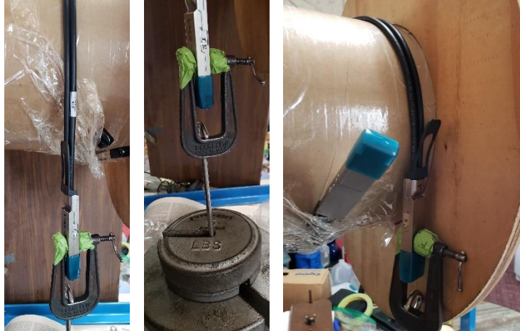
Figure 4 – Axial Cable Retention Test Setup
