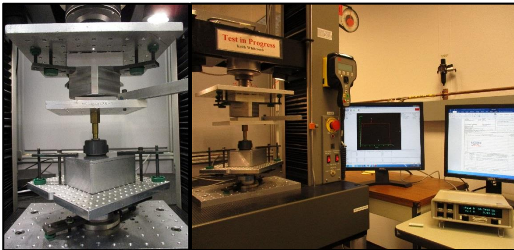
Figure 11 – Typical Receptacle Mounting Torque Test Setup
