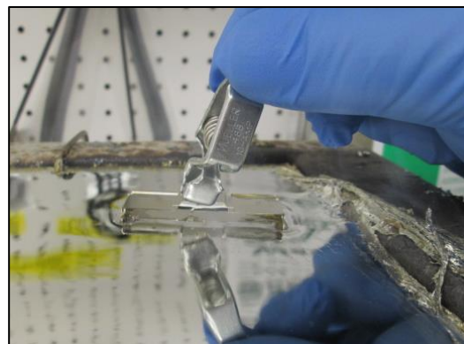
Figure 11 – Typical Solder Exposure
