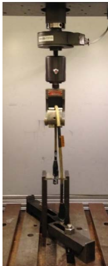
Figure 2 – Strength Test, Overmolded Connector
