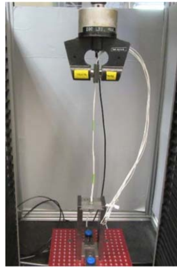
Figure 3 – Strength Test, Non-Overmolded Connector
