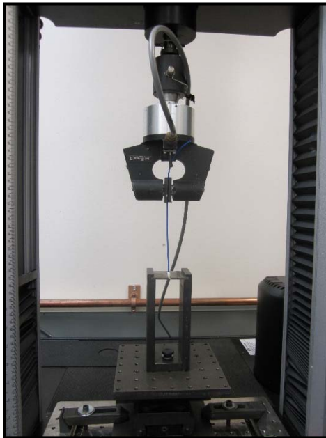
Figure 2 - Wire Retention Test Setup
