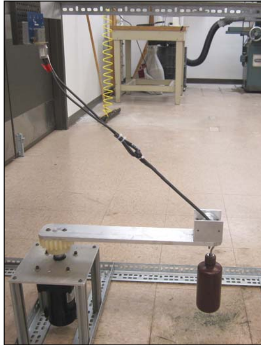
Figure 5 – Typical Test Setup, Rotational Cable Pull
