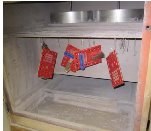
Figure 12 – Dust Test Setup
