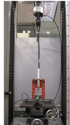
Figure 11 – Cage Latch Axial Retention Setup
