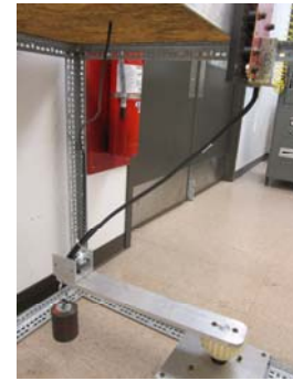
Figure 7 – Rotational Cable Pull Setup
