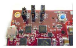
6. Turn on the power to the board with the switch next to the barrel jack. When the board powers up, the MicroZed will briefly illuminate a red LED, which will then turn off after less than a second. Once the FPGA has been successfully programmed by the boot image on the SD card, a blue "Done" LED will illuminate on both the MicroZed and the I/O carrier card. Your hardware should appear as shown below. If the board was powered on before this step, turn the power off and repeat this step.
