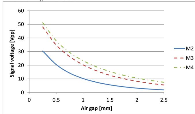
Typical sensor output voltage (peak-to-peak) for 15m/s
