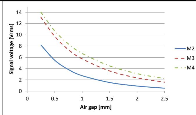
Typical sensor output voltage (rms) for 15m/s
