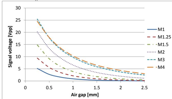
Typical sensor output voltage (peak-to-peak) for 15m/s
