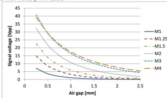
Typical sensor output voltage (peak-to-peak) for 15m/s
