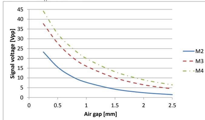
Typical sensor output voltage (peak-to-peak) for 15m/s
