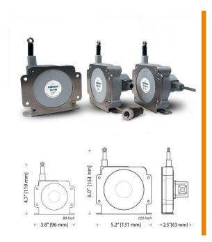
The SG1 provides absolute linear position up to a 10-ft. stroke range. Constructed with a rugged polycarbonate body, this model is available in an 80-inch or 120-inch stroke range and offers optional IP67 protection for wet or outdoor installations and an M12 connector for easy installation.
