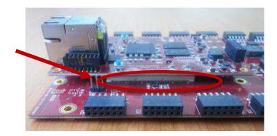
5. Connect the MS8607 digital pressure sensor to the "JC" Digilent Pmod™ port of the I/O carrier card, ensure that jumpers J1, J2, and J3 are configure such that the MicroZed will boot from the SD card on start up, and connect the power adapter to the barrel jack on the I/O carrier card (shown on the bottom). Finally connect the micro-USB cable to the micro-USB port of the MicroZed (shown at the top). The USB cable will facilitate UART transmissions for the console application.
