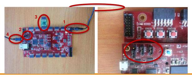
6. Turn on the power to the board with the switch next to the barrel jack. When the board powers up, the MicroZed will briefly illuminate a red LED, which will then turn off after less than a second. Once the FPGA has been successfully programmed by the boot image on the SD card, a blue "Done" LED will illuminate on both the MicroZed and the I/O carrier card. Your hardware should appear as shown below. If the board was powered on before this step, turn the power off and repeat this step.
