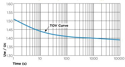
Temperature of samples (pre-heated): 60°C according to IEC 60099-4, Ed 2.0 2004. TOV Curve applies to an arrester which has a pre-stress applied prior to TOV verification. This prestress is equivalent to one high current impulse of 65 kA, 4/10 µs as per the switching surge operating duty test.
