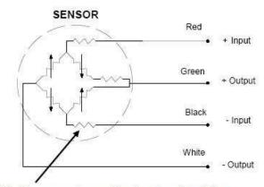
EPL-B0 compensation resistors in external module
