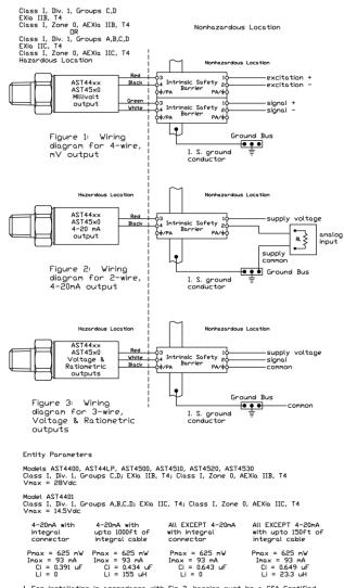
For installation in accordance with Fig 2, barrier must be a CSA Certified, Single Channel grounded Shunt-Blode Zener Barrier or a Single Channel Isolating Barrier.
