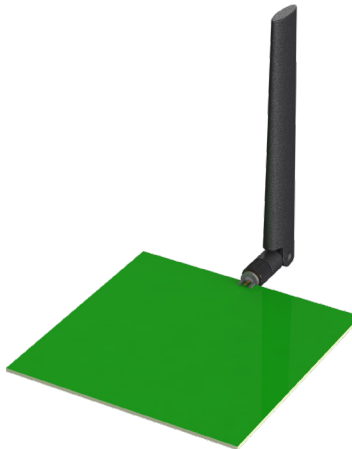
Figure 10. ANT-5GWWS3-SMA on Edge of Ground Plane, Bent 90 Degrees (Edge-Bent)
