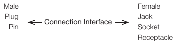
Figure 2. Typical RF Coaxial Connector Gender Terms
