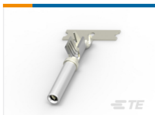
TE Part #2098253-2 SOC, SF, SIZE 16, 14-16 AWG, NI/SN
