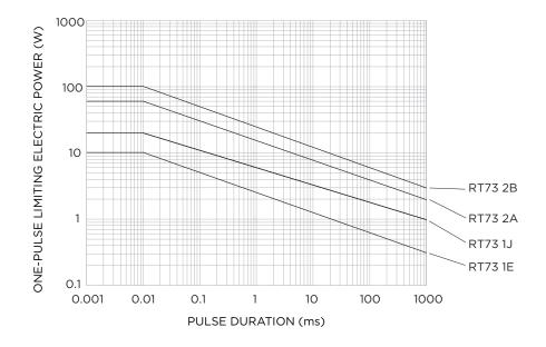
Note: For guidance only. The maximum applicable voltage is equal to the max. overload voltage. The pulse endurance values are not assured values, and it is recommended testing in the intended application.
