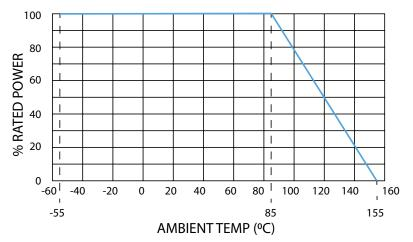
Note: For resistors operated at an ambient temperature of 85°C or higher, the power shall be derated in accordance with the above derating curve.
