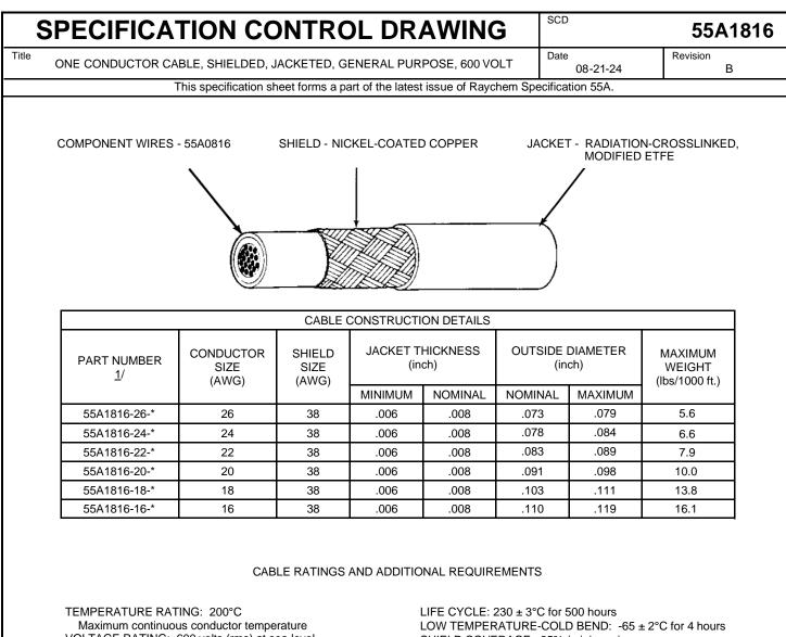
VOLTAGE RATING: 600 volts (rms) at sea level ACCELERATED AGING: 300 ± 3°C for 7 hours BLOCKING: 200 ± 3°C for 6 hours DIELECTRIC WITHSTAND: 1500 volts (rms), 60 Hz FLAMMABILITY: Procedure 1, 3 seconds (maximum), 3 inches (maximum); no flaming of facial tissue JACKET COLOR: White preferred JACKET COLOR: White preferred JACKET ELONGATION AND TENSILE STRENGTH: Elongation, 50% (minimum) Tensile Strength, 5000 lbf/in<sup>2</sup> (minimum) JACKET FLAWS:
