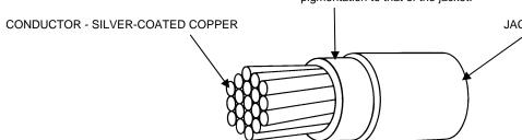
JACKET - RADIATION-CROSSLINKED, MODIFIED ETFE
