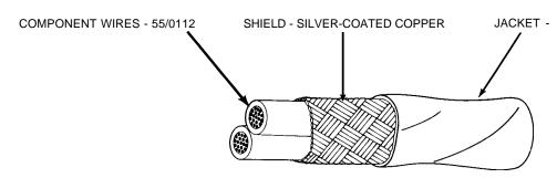
LOW OUTGASSING, RADIATION-CROSSLINKED, MODIFIED ETFE
