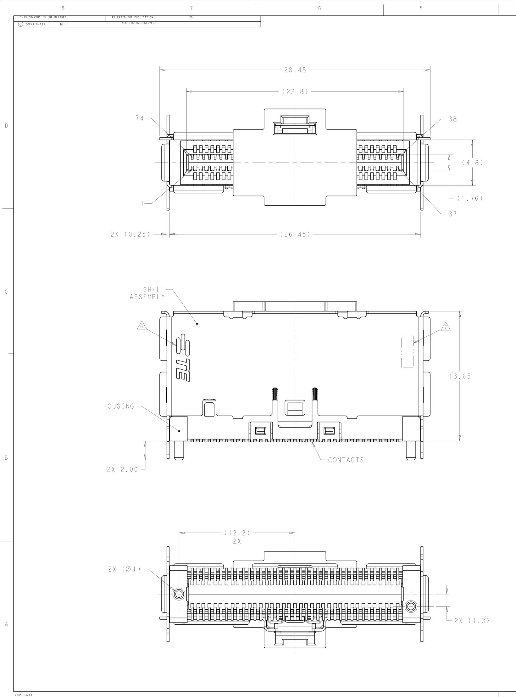
A HOUSING AND CONTACT OVERMOLD: LCP, BLACK, UL94 V-0 RATED CAP: LCP, BLACK. Contacts: copper alloy.
