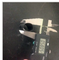
INCORRECT OD TUBING IS COMPRESSED INTO AN OVAL SHAPE
