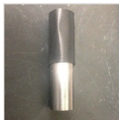
CORRECT ID PLUG GAGE KEEPS TUBING ROUND
