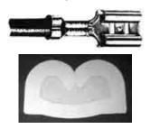
The standard crimp on all straight and certain flag type FASTON terminals is the "F" crimp. Experience over widespread segments of the industry has proved this crimp the most effective way of providing stable electrical and mechanical performance. Applied with match-mated tooling, the "F" crimp offers the optimum combination of mechanical strength and electrical conductivity. This method of termination also provides maximum resistance to vibration and corrosion.
