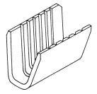
This crimp is designed for reliable, high-speed connection of magnet wire. The conductor(s) is automatically multiple-ring stripped and forced into sharp serrations with a single precision-controlled solderless crimp. This operation produces a strong, air-tight termination that is as resistant to corrosion and many other environmental effects as the insulated conductor itself.
