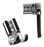
In making this crimp, a tab on the wire barrel, is inserted through a slot in the terminal itself. The crimping action is continued by flattening the tab between two lances which in turn are locked over the tab. The wire connection is locked in to offer reliable electrical and mechanical performance. This receptacle design includes a lance-tab stop at its rear to avoid over-insertion of shoulderless tabs. The "C" Crimp
