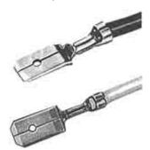
The wire crimp tabs are designed for line splices and other special applications. They can be applied to 22-14 AWG wire with "F" crimp termination and include insulation support. The wire crimp tab is also available with AMPLIVAR connector type serrations for magnet wire applications.
