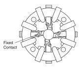
Contacts Shown With Coil 1-2 De-Energized and Coil 3-4 Energized.
