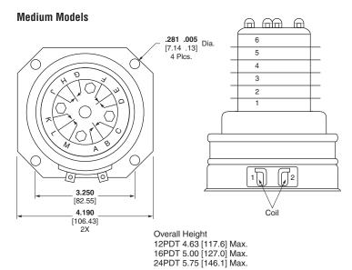
Coil and Contact Terminal Screws #5-40 Supplied.
