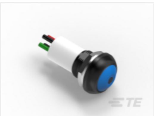
TE 产品编号2-2329388-5 PB OFF/ON FC BLU M1 TERM BLU LED IP68 50
