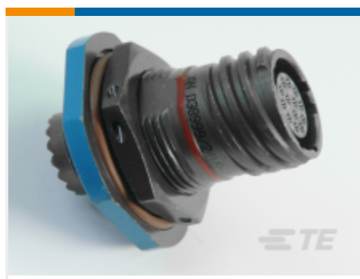
TE 产品编号 CAT-D38999-DTS10X D38999: Jam Nut, 23-55 Insert, Electroless Nickel Plating
