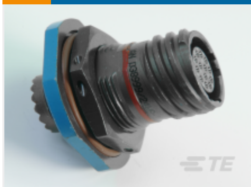
TE 产品编号YDTS24F25-35PAV001 D38999: Jam Nut, 25-35 Insert, Electroless Nickel Plating
