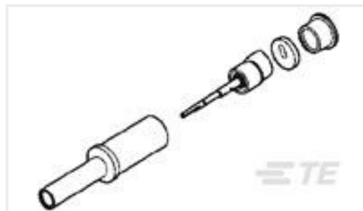
TE 产品编号1757624-1 SZ 8 COAX PIN,RG142,HEX CRIMP
