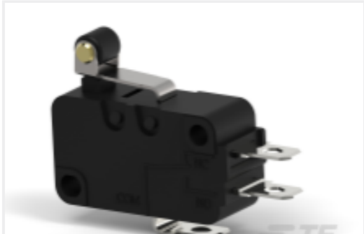
TE 产品编号2351459-1 SMINSA SW SH-H-R 0.49N. 5A AC DT SLD
