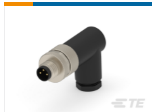
TE 产品编号T4013008031-000 M8, SCREW, MALE, R/A, UNSHIELD, 3P, GOLD
