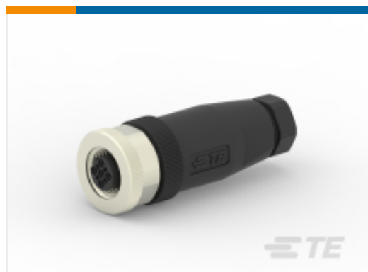
TE 产品编号T4110401031-000 M12,FEMALE,STRAIGHT,B CODE,3P, PG7,GOLD
