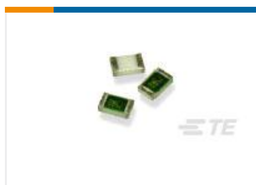
TE 产品编号1-1614885-8 CPF 0805 390K 0.1% 25PPM 1K RL
