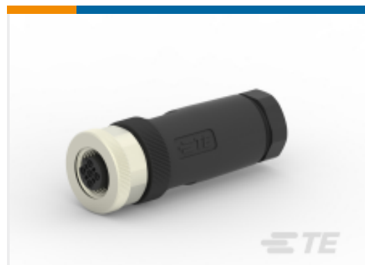
TE 产品编号T4110402051-000 M12,FEMALE,STRAIGHT,B CODE,5P, PG9,GOLD
