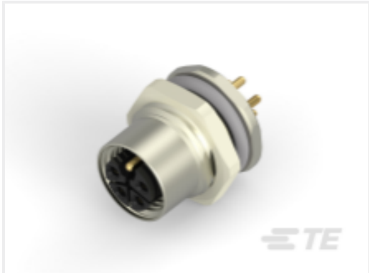
TE 产品编号T4141L12051-001 M12,REAR MT,F,L,4P+PE,LONGER, SOLDER PCB
