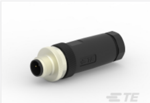
TE 产品编号T4111002021-000 M12,MALE,STRAIGHT,A CODE,2P, PG9,GOLD
