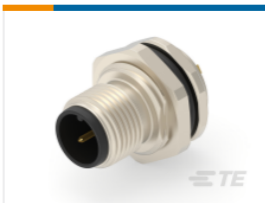
TE 产品编号T4130012021-000 M12,REAR MOUNT,MALE,A,2P, SOLDER WIRE
