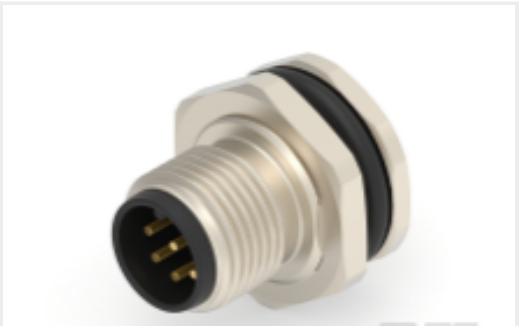
TE 产品编号T4130012081-000 M12,REAR MOUNT,MALE, A,8P, SOLDER WIRE
