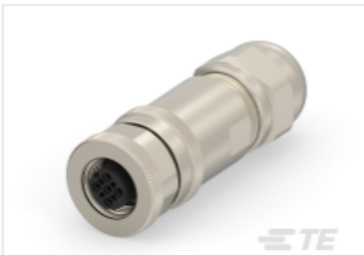
TE 产品编号T4110012051-000 M12 F, 5P GOLD A_CODE S SHIELDED PG9
