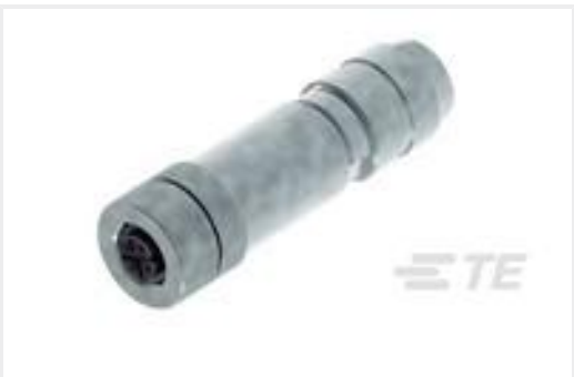
TE 产品编号6-2271117-2 M12,FEMALE, A CODE,12P,PG9, SHIELDED(AU)
