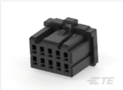
TE 产品编号CAT-D9934-A15B Receptacle and Tab Housing: 2.5 mm Pitch, 250V
