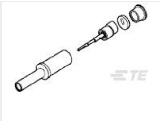
TE 产品编号1757624-1 SZ 8 COAX PIN,RG142,HEX CRIMP
